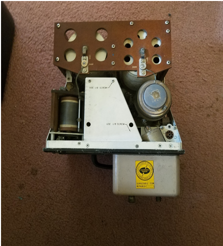
Remote Antenna Tuner
