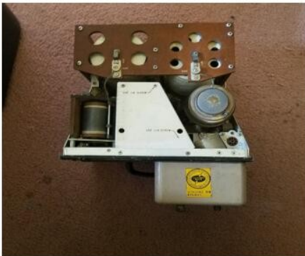
Remote Antenna Tuner
