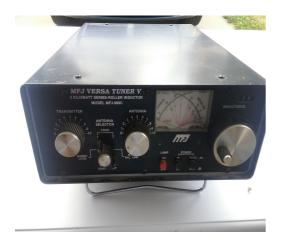
MFJ-989C Antenna Tuner 3KW MFJ-989C Versa Tuner V Frequency Range: 1.8 to 30 Mhz Cross-needle SWR/Power Meter Has forward power ranges 200 To 2,000 watt. Back Panel Outputs: 2 Coaxial Cables, 1 wire or balanced Line and 1 Dummy Load
